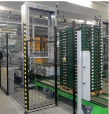
The Turning-cross (1) rotates the product according to the layer pattern required. With this feature, labels can be turned to the outside of the pallet if required, so that they are visible
